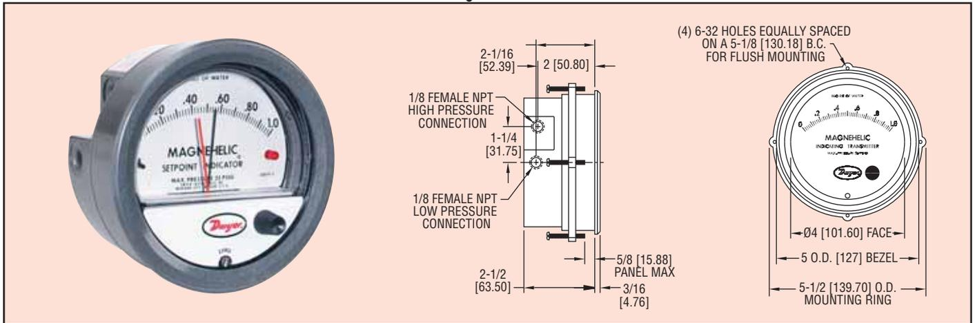
Bright red LED on right of scale shows when setpoint is reached. Field adjustable from gage face, unit operates on 12-24 VDC. Requires MP or HP style cover and bezel.
